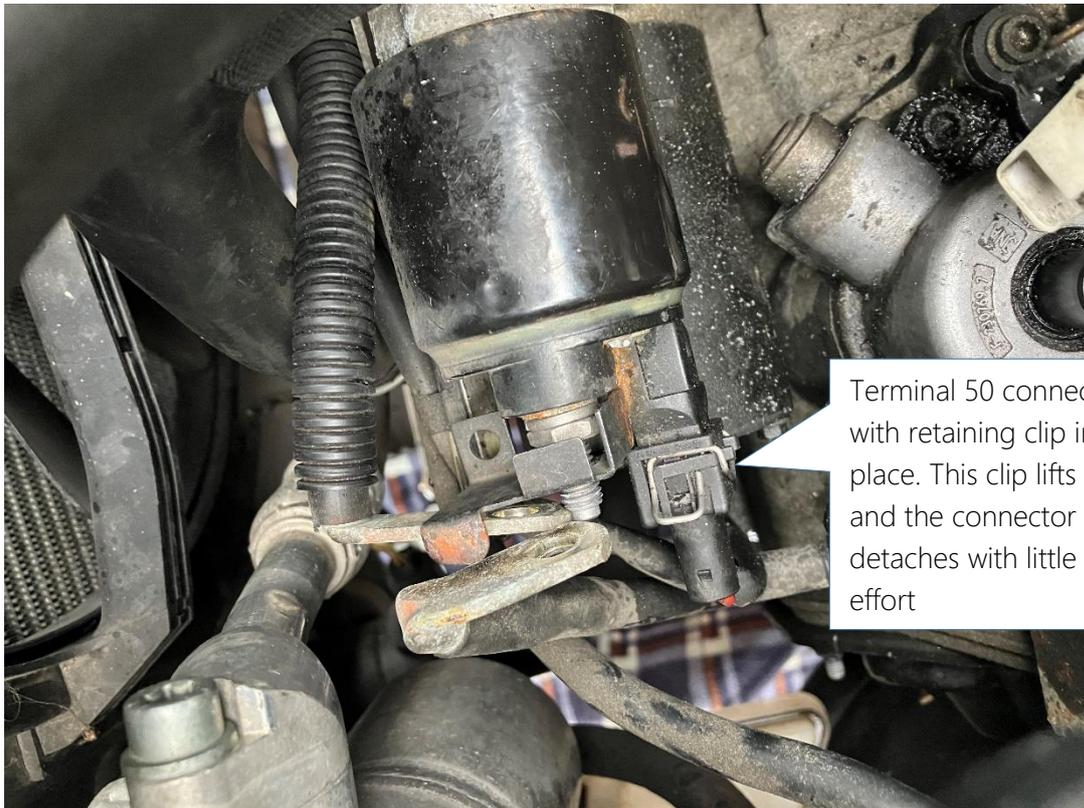
8. Next remove the lower starter motor bolt. I have shown this in an earlier picture in item 5. The nut that holds the protective cover in place has already been removed and you will need to slide a connector mounting bracket off the bolt to fully expose it. To remove the connector bolt you will need an 18mm socket.
