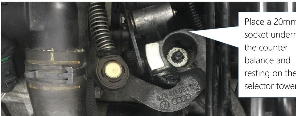
Place a 20mm socket underneath the counter balance and resting on the selector tower
