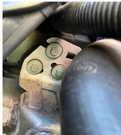
4. Next up you need to remove the gear selector linkage counter balance from the selector tower. This is held in place by a nut and will require a 13mm socket to remove. With this nut removed, all the videos I found showed sharp yanking upwards on the counter weight would release this from the splines. Despite 2 weeks of spraying with PB Blaster this was having none of it!
