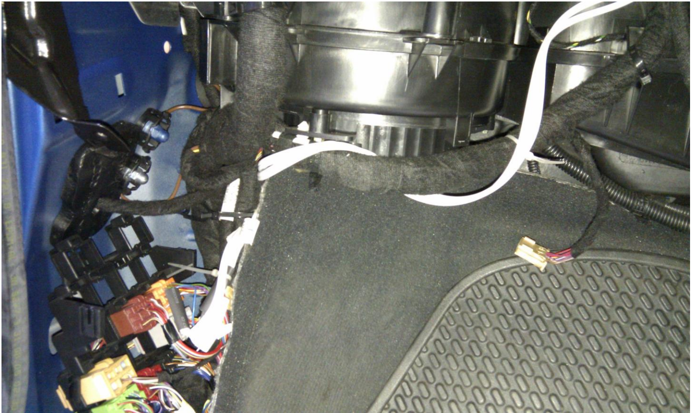
Wires routed (White speaker cable), soldered and connected to microphone wires in Orange connector.
