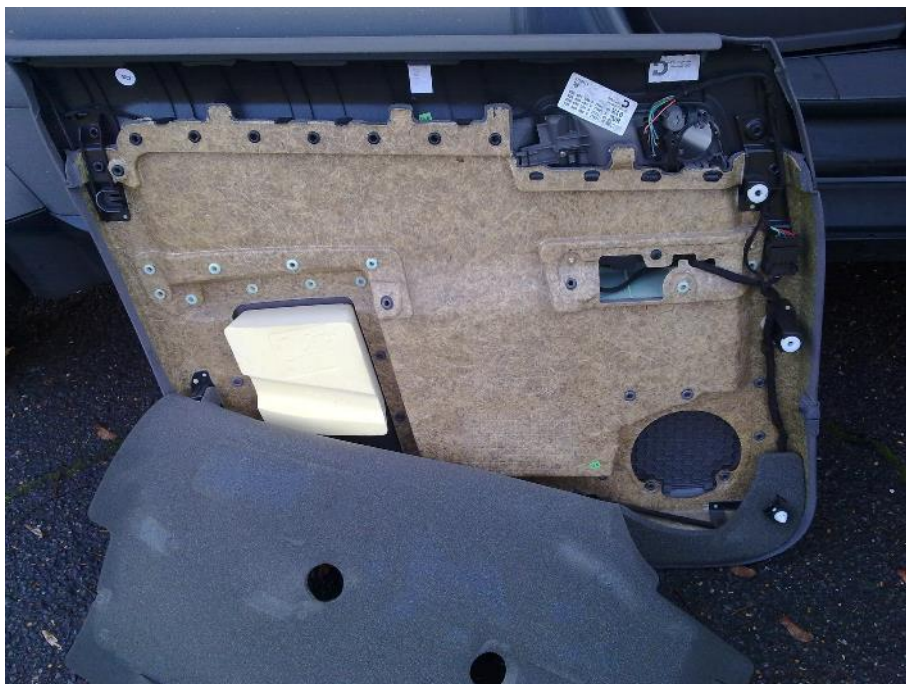
Step 5b Removing the trim backing
