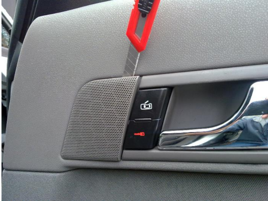
Step 1 - Removing Speaker Grill
