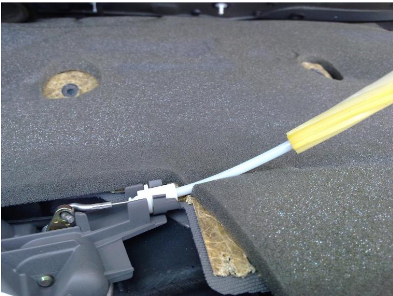
Step 2b Unclipping the door cable
