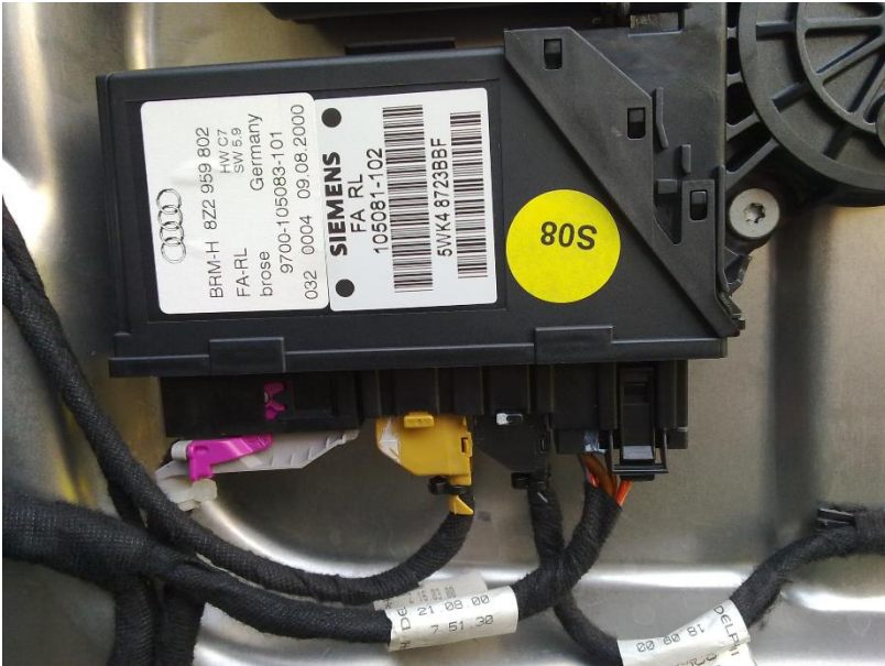
Step 4a unplugging the wiring loom
