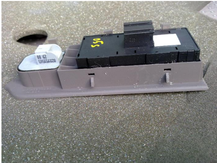
Step 6b Removing the windows and mirror swicht array
