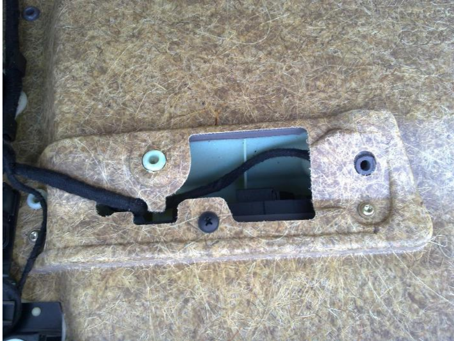
Step 6a Removing the windows and mirror switch array
