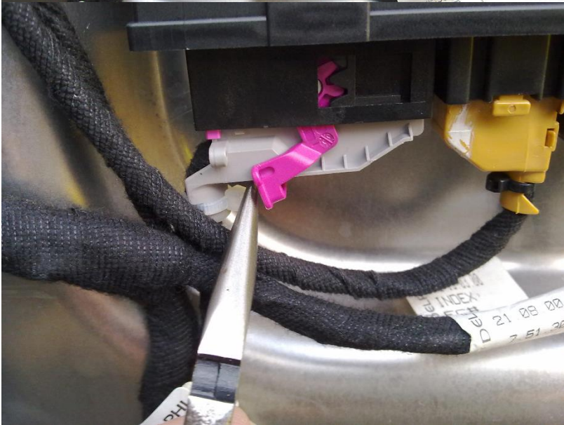
Step 4b unplugging the wiring loom
