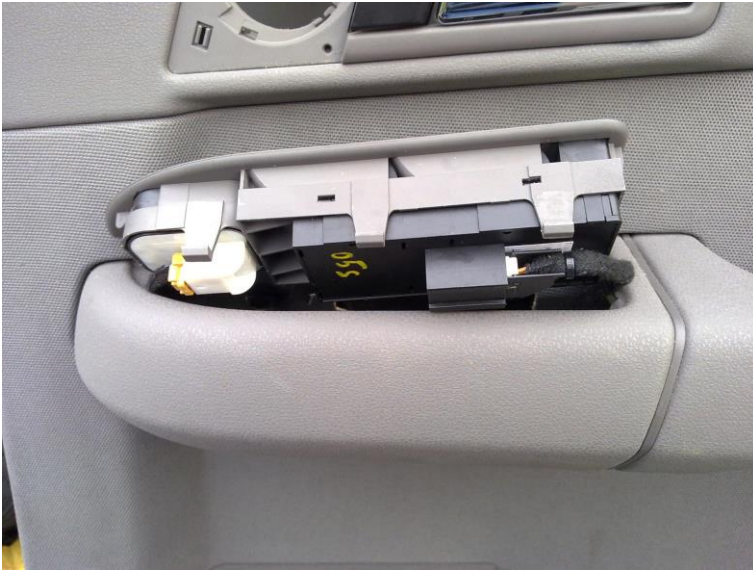
Step 9a Refitting the windows and mirror switches array
