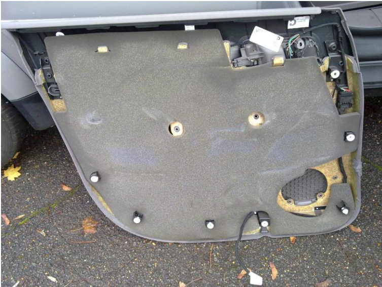
Step 9b Refit the plastic foam
