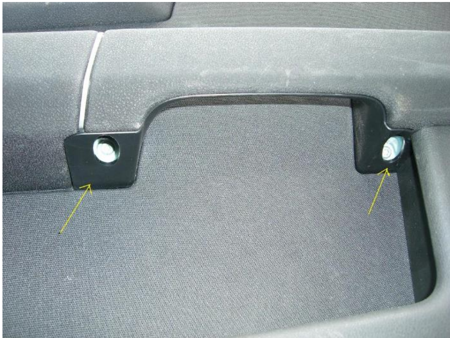
Remove 2 screws under door handle
