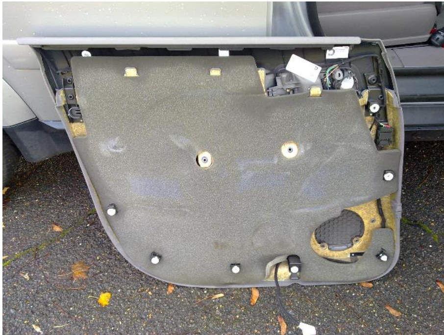
Step 5a Removing the trim backing
