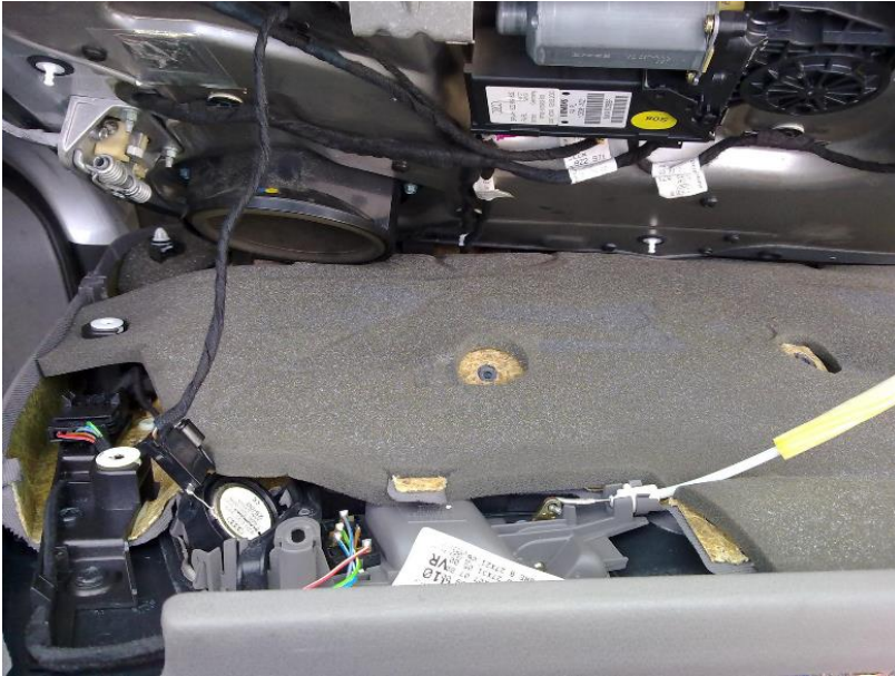
Step 2a Removing the Door Trim
