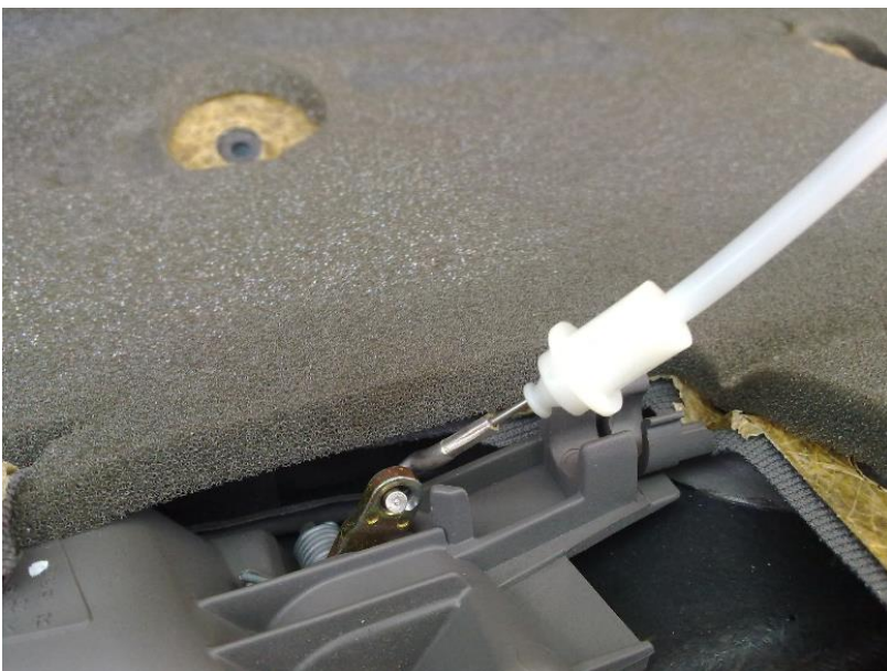
Step 2c Unclipped cable
