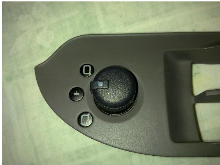
Step 8b Reassembling the windows and mirror switches array
