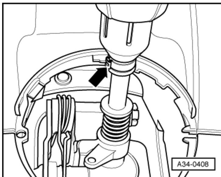
→ **Fig.4 Detaching and assembling cover ring and gear stick cover**
