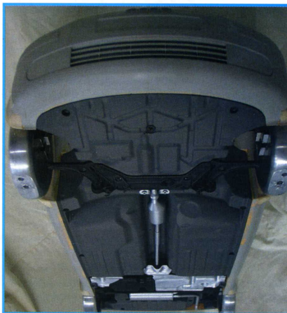
Under floor tray reduced drag
