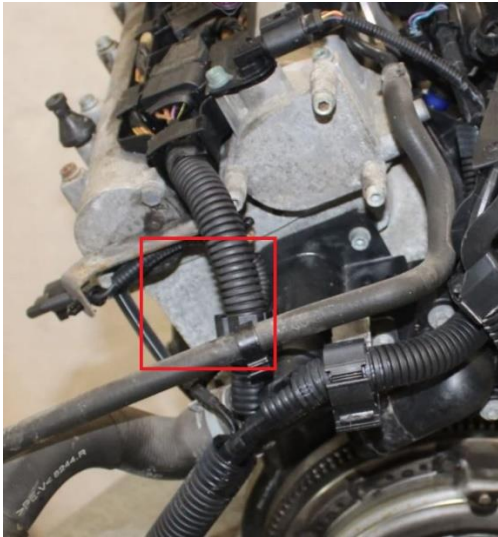
Picture shows a late BKY engine without outlet for the EGR valve.
