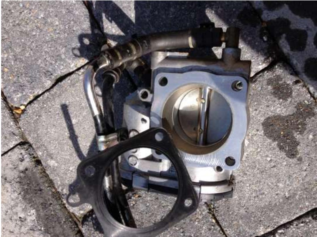
Now back to fitting, it's basically the reverse of removal, fit the new gasket and the clean throttle body back to the car
