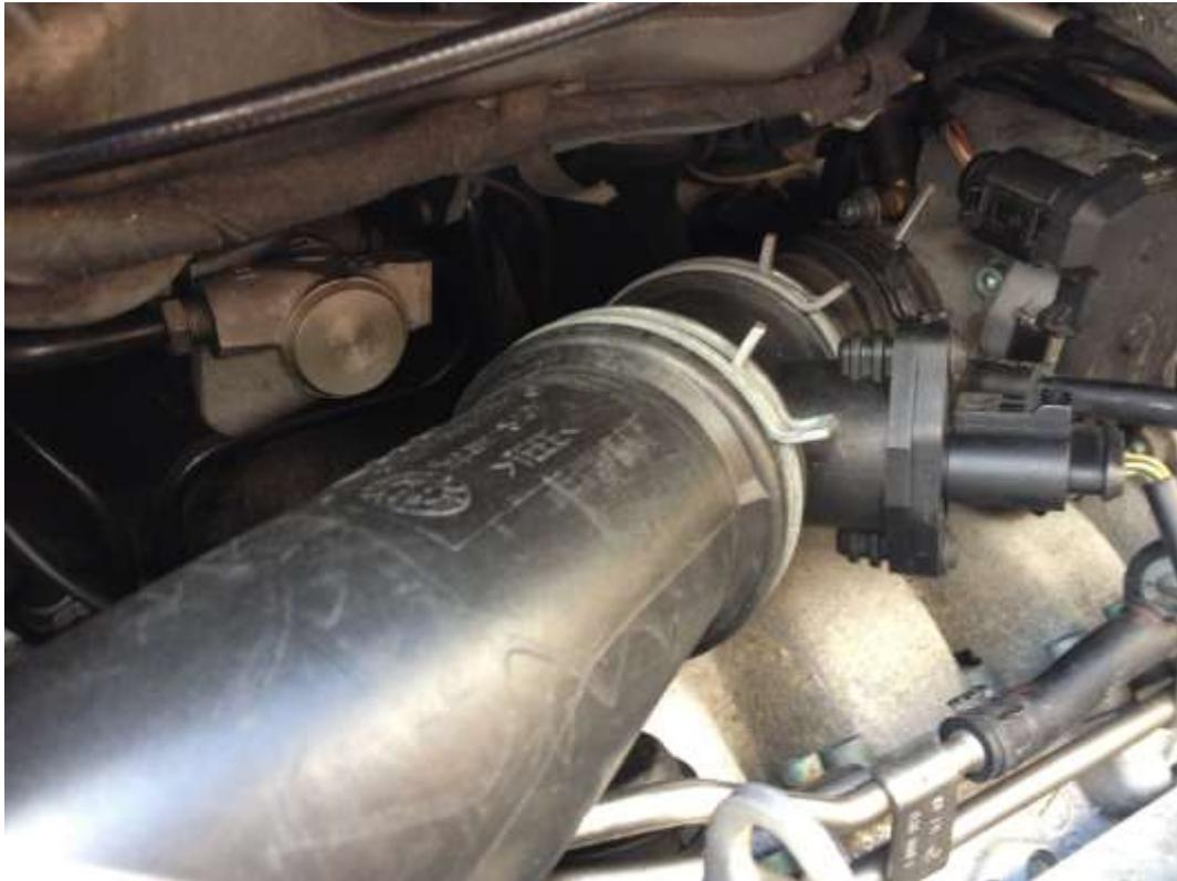
Now remove the plug to the MAF and remove it
