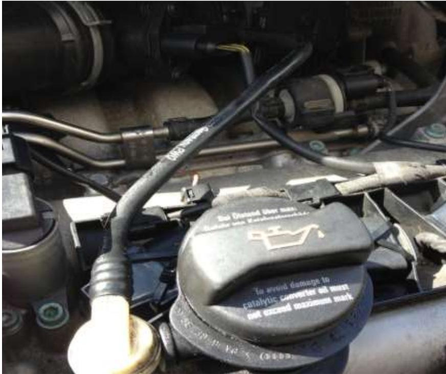
You should now remove the two water pipes and the bracket holding them on the side, to do this use a 10mm socket, and plug the ends of the water pipes to avoid leaking.
