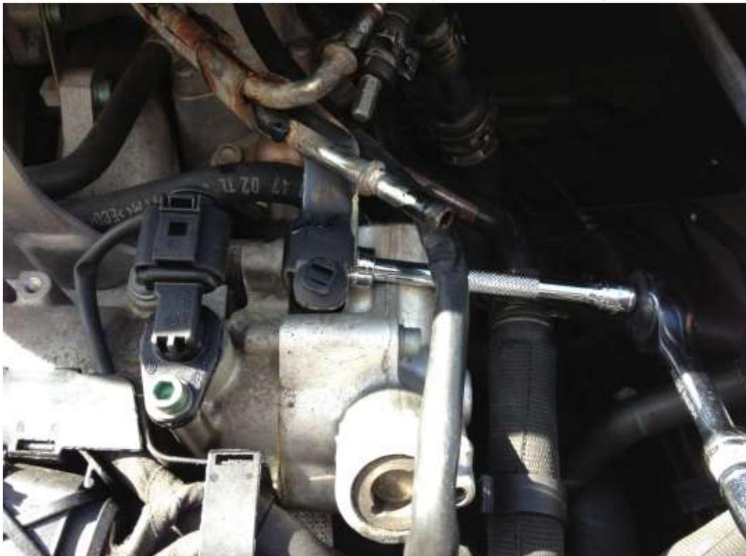
Now you should be able to remove the throttle body and start the cleaning process.
