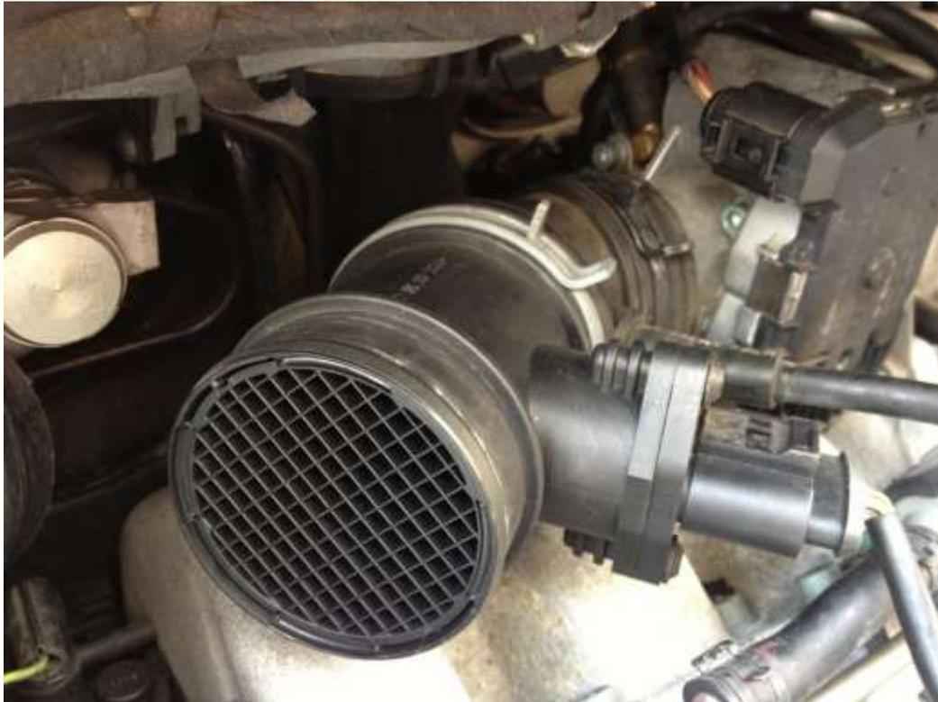
With the MAF and initial pipe removed all you have left is one curved pipe with the oil breather attached, remove this and oil breather from the engine
