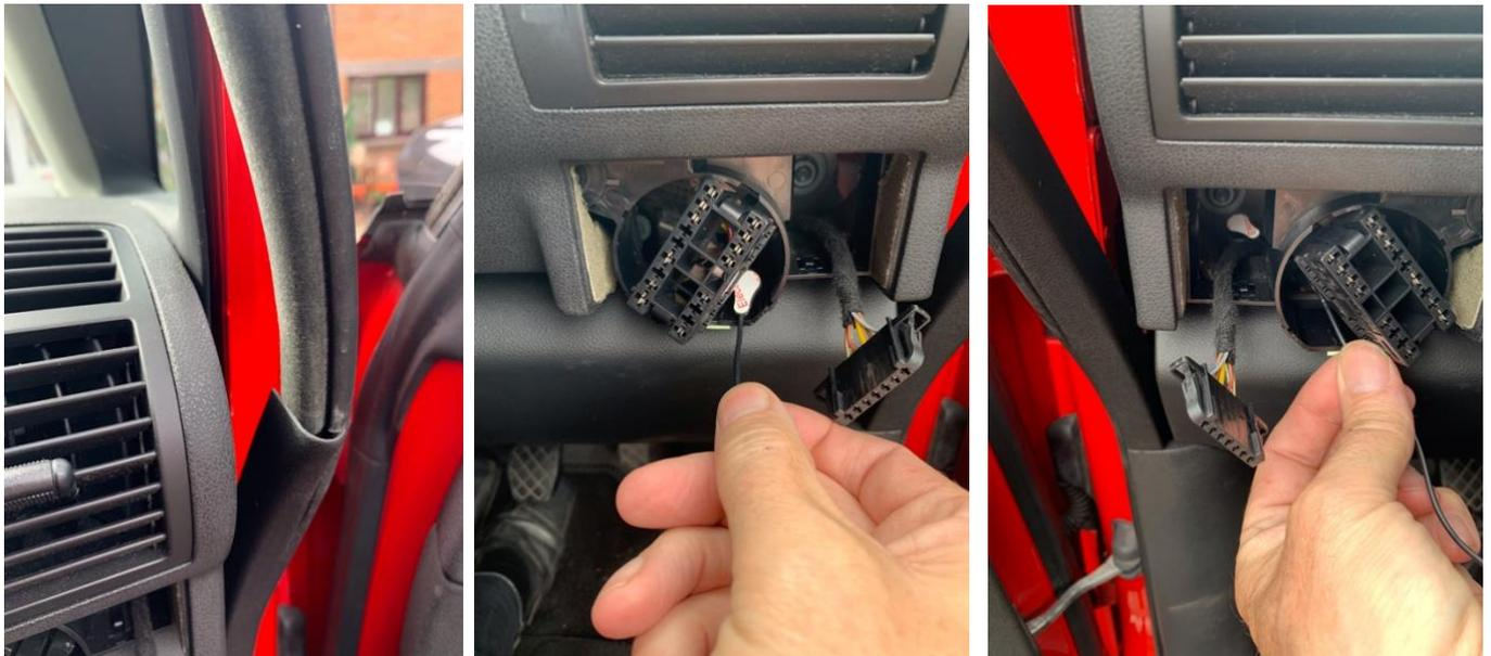
Take up the excess wire into a bundle and then feed it through and reinsert the fascia. Tap back the door seal, remove the backing from the sensor and stick in position. I actually use mine in the triangular window to keep the wiring simple.
