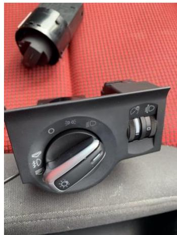
Now we need to replace the unit but firstly we need to feed the sensor through the hole where the switch goes so that the wiring is not trapped. To prepare for the routing of the sensor depends on where you want to position it. It works fine anywhere you want to put it but I prefer a short and easy route, although some people might prefer to feed it to a point behind the instrument cluster cowling. It is up to you. But me being a bit lazy I prefer the following option.
