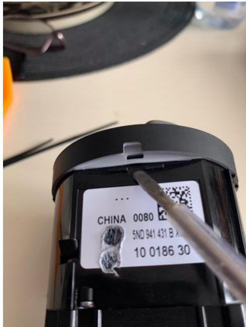
This will loosen the icon ring but the hole in the centre is not big enough to allow you to remove it. To get it off you need to remove the Brushed Aluminium section of the knob. You need to use a fair amount of force but work on one side until it is free then the other. The trim will then lift up and slide off
