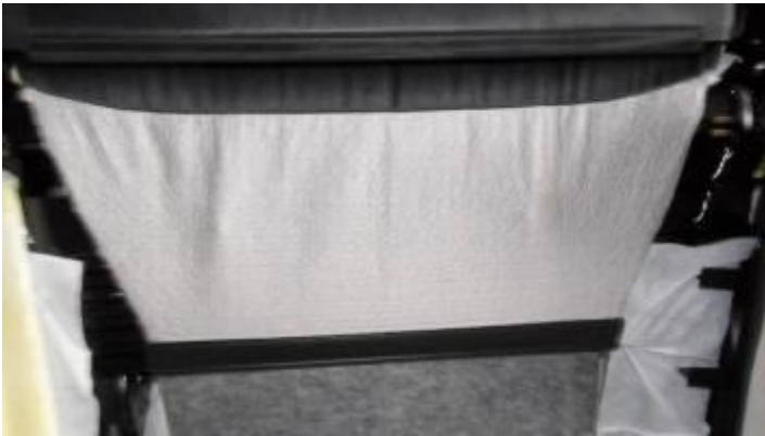
Next , prise the felt backing away from the metal plate. It is a U shaped plastic clip.
