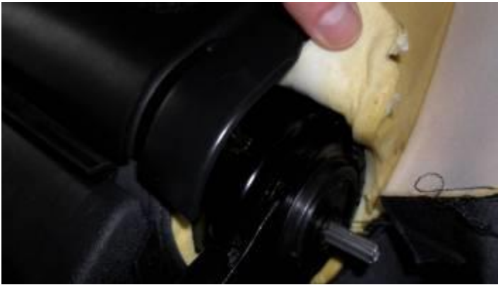
Once released, the plastic backing can be lifted away from the seat.
