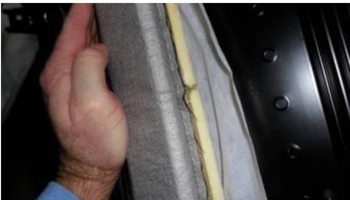
Next , prise the felt backing away from the metal plate. It is a U shaped plastic clip.
