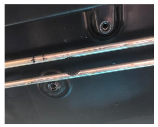
After removing the original motor mount, the new one should be fitted as seen here. Make sure all the countersunk Allen bolts are tight, when they are, the mount pieces should touch, and the tubes should be tightly clamped within the mount. Screw the short, non-countersunk Allen bolt into the hole shown in the bottom left of this photograph.
