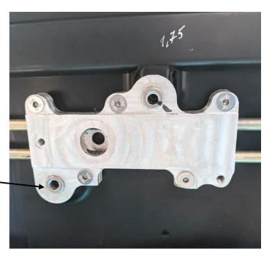
Screw the last remaining Allen bolt through the motor, and into the rear-most hole of the motor mount, as shown.
