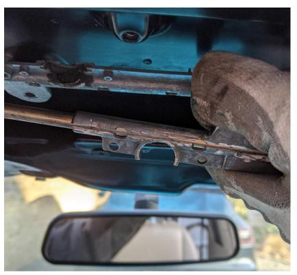
With a sharp grinding disc in a Dremel, the cutting will happen relatively fast, be careful not to cut into the bronze coloured tube, as this could damage the cables inside.
