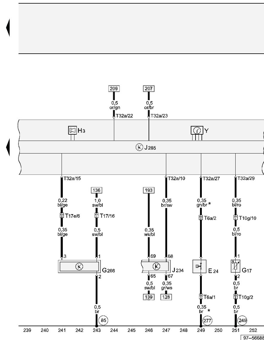
Belt switch - driver's side, ambient temperature sensor, oil level/oil temperature sender, airbag control unit
